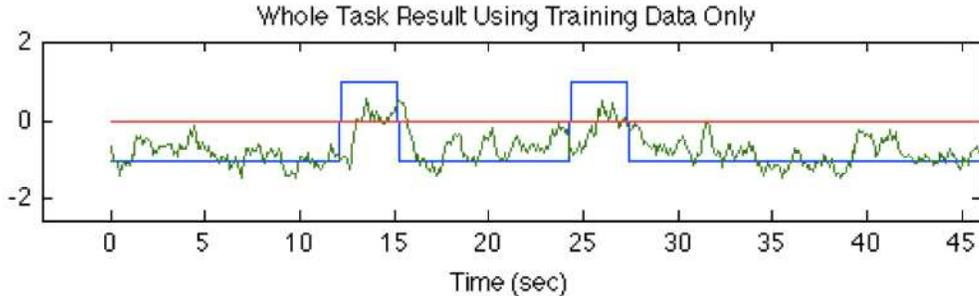
Figure 1: Classification by using the PSVM. The green line is the classifying attempt (i.e.  $x^T w - \gamma$ ). The blue line is  $-1$  when the cue under observation has not been cued and  $+1$  when the command is cued. The red line is  $0$ . Hence, when the green line is above the red line, we classify that data point as the action having occurred. Otherwise, we classify the data point as the action not having occurred.
